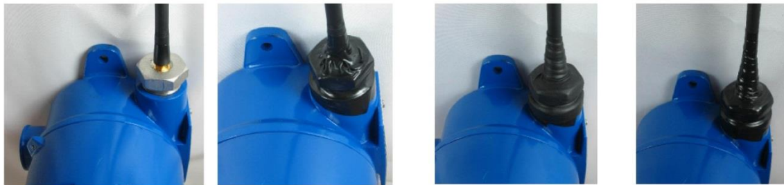
Figure 14 Water-proofing Antenna Connections
