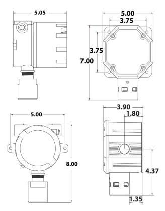
Figure 1 Mounting Dimensions
