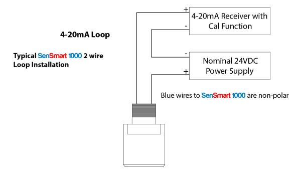
Figure 2 SenSmart 1100 Wiring
