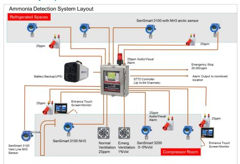
fan. Others should be spaced in the breathing zone about 5 feet above the floor every 2000 sqft. The 0-5% detector should be located 5 feet above the floor and below the emergency ventilation fan. It should activate the EV fan (1% alarm trip) and also shut down compressors, pumps and disconnect power sources (2% alarm trip).
