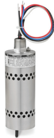
Diffusion "Smart" Sensor with Splash Guard and Cal Port
